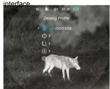
Press the Up (6) / Down (3) button to select Zeroing Profile and briefly press the Menu (4) button to select the Zeroing Profile.
